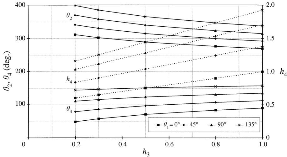
FIGURE 14. Variations of the angles  $\theta_2$  and  $\theta_4$ , and the thickness  $h_4$ , versus  $h_3$  for different angles of incidence  $\theta_1$ .
