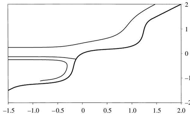
FIGURE 10. Impact of a jet of width 0.5 on a wall. The shape is given by two sinusoidal periods with wavelengths of 2 extended by two plates and is inclined at an angle of  $45^\circ$ .
