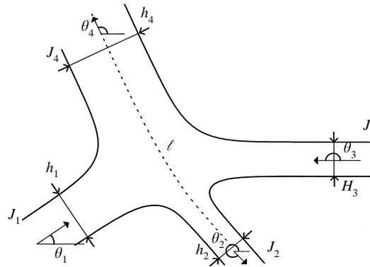
FIGURE 1. General configuration of two impinging free jets.
