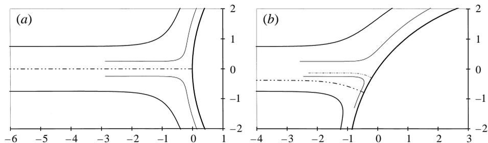
FIGURE 8. (a) Impact of a jet of width 0.5 and 1.5 at normal incidence on an arc of parabola extended by two plates. (b) The wall is rotated by an angle of  $35^\circ$ .
