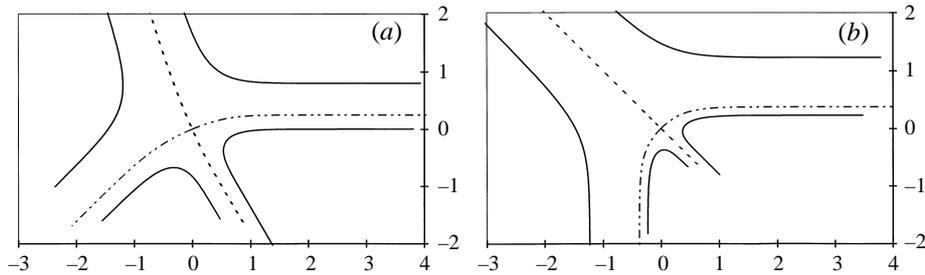
FIGURE 15. Impinging free jets. (a)  $\theta_1 = 0^\circ$ ,  $h_1 = 1$ , and  $h_3 = 0.5$ , (b)  $\theta_1 = 90^\circ$ , and  $h_1 = h_3 = 1$ .
