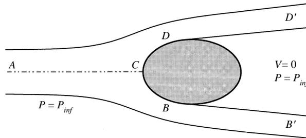
FIGURE 5. Jet impinging on an obstacle.
