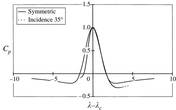
FIGURE 9. Pressure coefficient distribution along the two barriers for  $h_A = 1.5$ .
