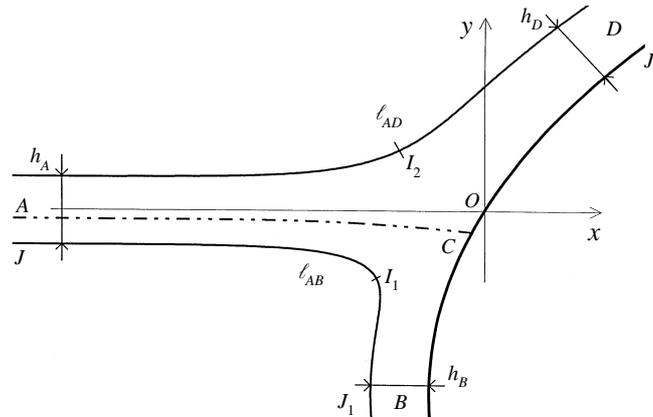
FIGURE 4. Jet impinging on an infinite wall.
