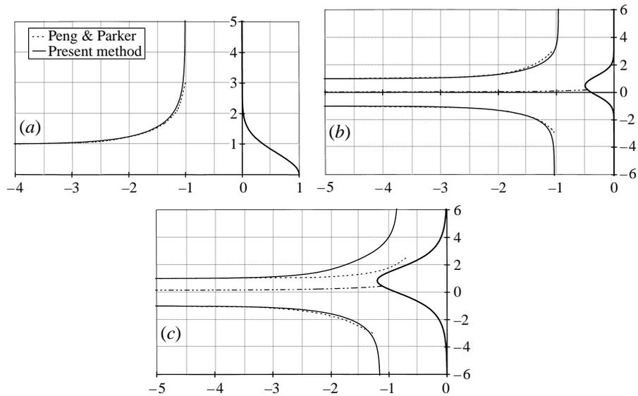
FIGURE 7. Impact of a jet of width 2 at normal incidence on symmetric and asymmetric walls: (a)  $x(y) = e^{-y^2}$ , (b)  $x(y) = -0.25e^{-(y-0.2)^2}$ , and (c)  $x(y) = -1.2 \operatorname{sech}(y - 0.85)$ .
